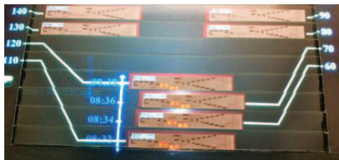
Figure 4: tangible computation of an arrival sequence: allocation within projected time slots (blue), computed stack exit times (red), strips linked to their projected stack level (white - crossing links show a misordering). This was inspired by a kind of paper ruler that is used by Orly approach controllers as rough paper that helps visualize free time slots and calculate mentally (Fig 6).
