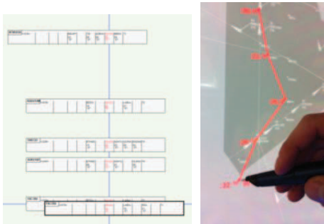
Figure 7: a) a timeline representing several flights heading to a common beacon to analyze potential conflicts; b) computation of the time needed for the drawn trajectory. The controller draws a polyline with the pen onto the radar screen where the estimation of time and distance to reach it is displayed next to the related nodes.
