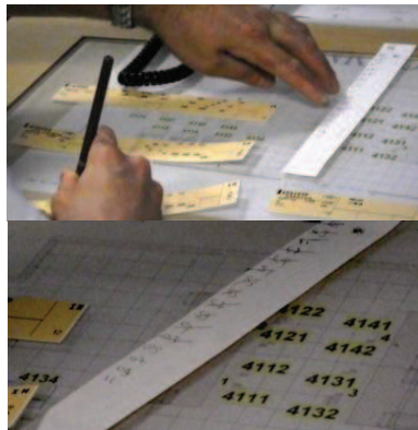
Figure 6: a) a rough paper ruler on the back of a strip to allocate an arrival sequence; b) the paper ruler contains stack exit times as mentally computed by the approach controller.
