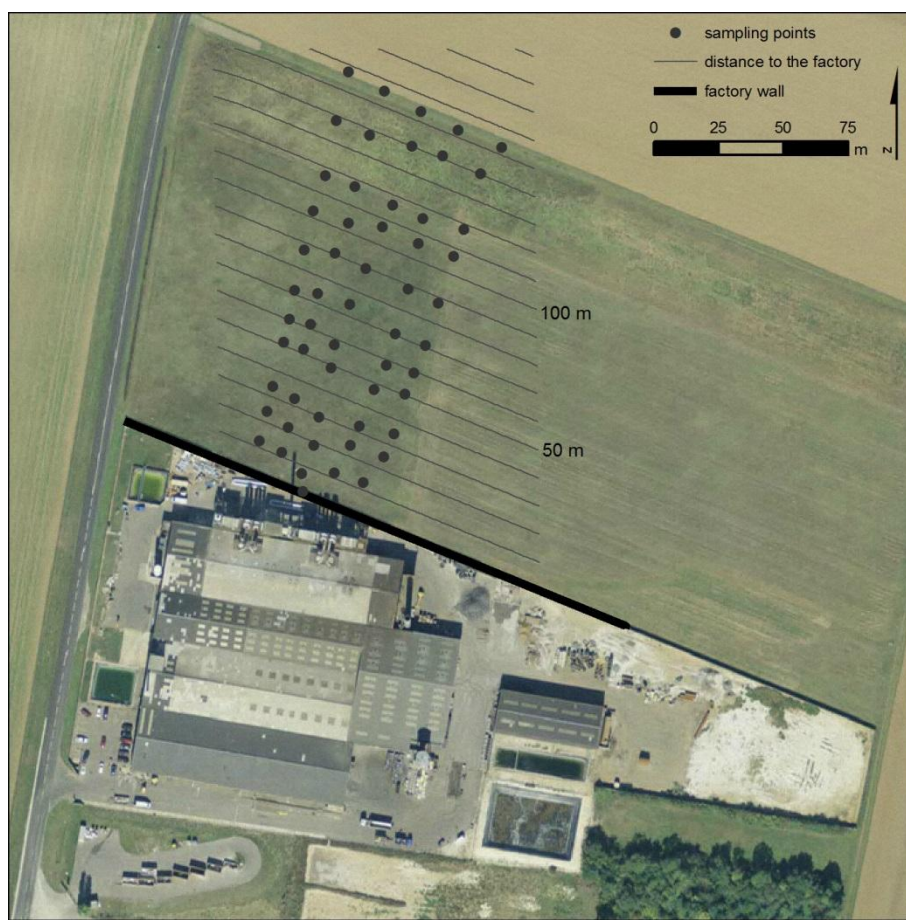
Figure 1: Map of the study site: lead recycling smelter in Bazoches-les-Gallérandes and the experimental plot. The sampling strategy is drawn by the five transects from 10 to 150 m to the smelter courtyard.
