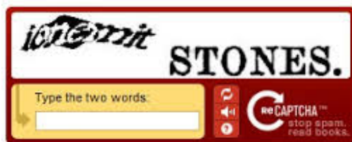
Figure 2.4: The ReCAPTCHA user interface. The left word is computer generated and the right word is extracted from a book to be digitalized.
