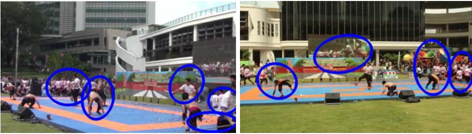
Figure 3.19: 2D elliptic ROIs, as computed in Step (1) of our algorithm, on the RagAnd-Flag dataset.
