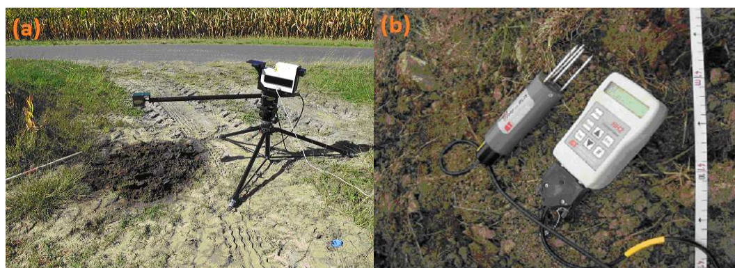
FIGURE 4.2 – (a) SVC Spectroradiometer for bare soil spectral sampling (b) ML3 Theta-Probe for soil moisture measurements.
