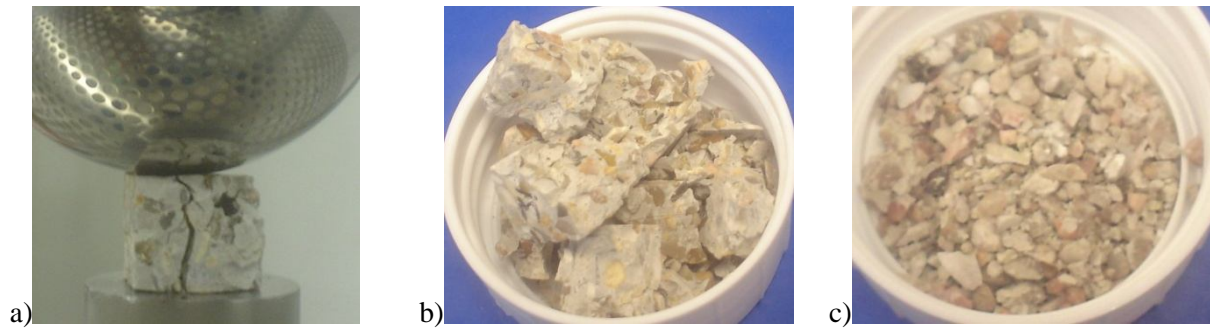
Figure 5.11. HPB fracture of concrete cubes showing a) Concrete cube displaying fracture mode indicative of a vertical plane of high tensile stress b) Fragments of untreated concrete samples after HPB impact. Concrete samples remain largely intact as 2-3 large fragments and c) Fragments of a long microwave treated concrete sample after HPB impact. Fragments are very small and the largest are mostly liberated aggregate
