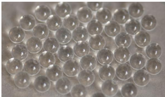
FIGURE 1. 6mm soda lime glass beads used for single-particle impact testing on a Hopkinson bar
