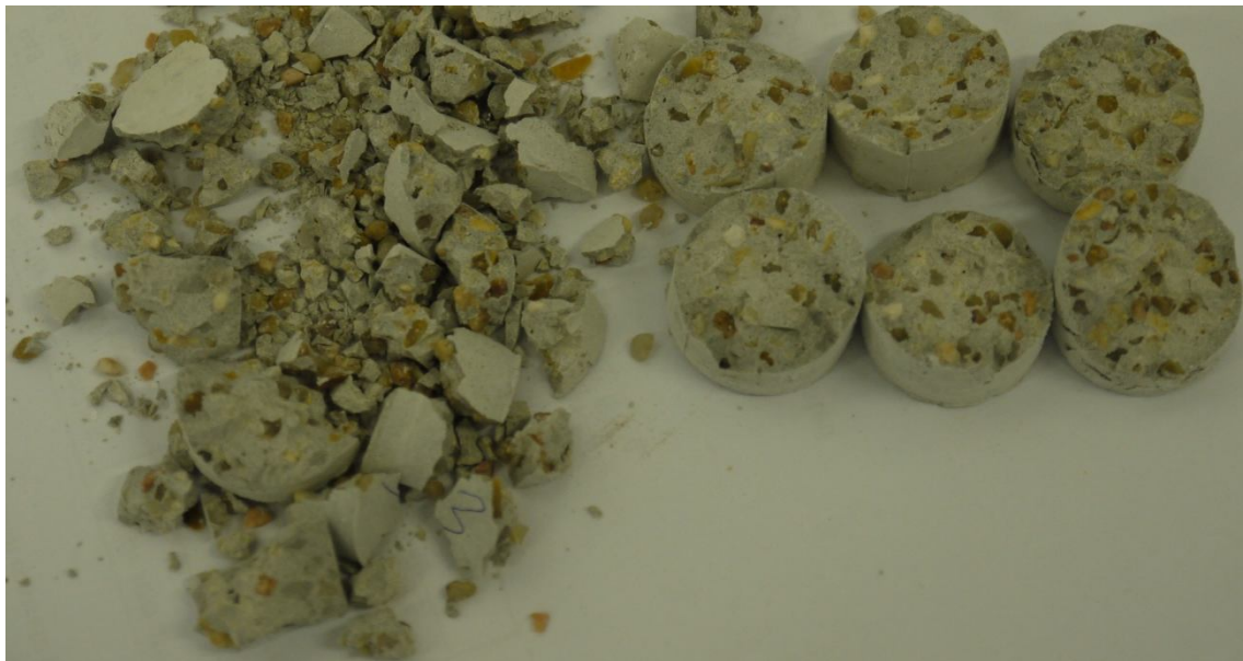
Figure 5.27. Concrete samples that have experienced microwave heating induced spalling
