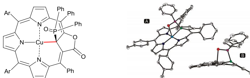
Figure 51: Schematic view and X-ray structure of a copper(II) complex bearing a weak Cu-C bond (from reference 226).
