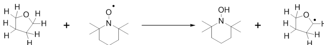
Figure 84: Putative reaction of THF and (2,2,6,6-Tetramethylpiperidin-1-yl)oxyl (TEMPO) to give TEMPO H and tetrahydrofuryl radical.
