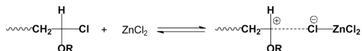
Scheme 5: Exchange process between the HCl–vinyl ether adduct and the carbocation discovered by Sawamoto and coworkers (reference 34).
