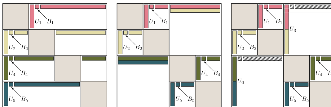
(a) First step of row compression at the leaf level l . The blockrows U_1 B_1 , U_2 B_2 , U_4 B_4 , and U_5 B_5 are entirely compressed. (b) Second step of row compression level (parents of the leaves). Matrices generated through compression at previous level are partly merged. (c) After the merge, blockrows U_3 and U_6 are recompressed.
