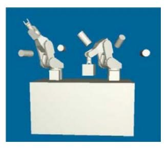
Figure 3.11: From [45]: Path planning for a dual-manipulators system with 12 DOFs in changing environments.
