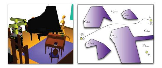
Figure 2.2: From [17]: a) A Piano Mover's Problem. Two robots and a virtual character cooperate to transport a piano in a workspace  $\mathcal{W} \subset \mathbb{R}^3$ . b) The configuration space is divided in  $\mathcal{C}_{free}$  (light areas) and  $\mathcal{C}_{obstacle}$  (dark areas). A path can be found between  $\mathbf{q}_1$  and  $\mathbf{q}_2$  because they lie in the same connected component of  $\mathcal{C}_{free}$ , which is not the case for  $\mathbf{q}_3$ .
