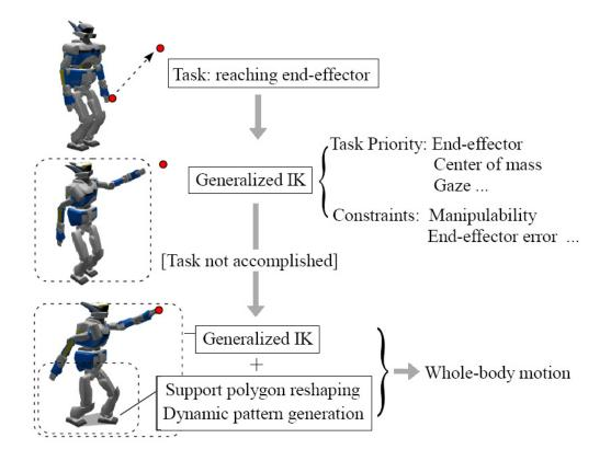
Figure 6.3: From [70]: GIK: A general framework for task-driven whole-body motion including support polygon reshaping.
