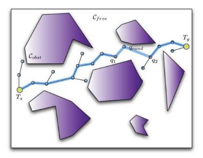
Figure 2.4: From [17]: With the RRT algorithm, two trees rooted on  $\mathbf{q}_{init}$  and  $\mathbf{q}_{goal}$  can be grown simultaneously. Each tree is extended until leaf configurations  $\mathbf{q}_1$  and  $\mathbf{q}_2$  from each tree can be connected by a randomly drawn configuration  $\mathbf{q}_{rand}$ .
