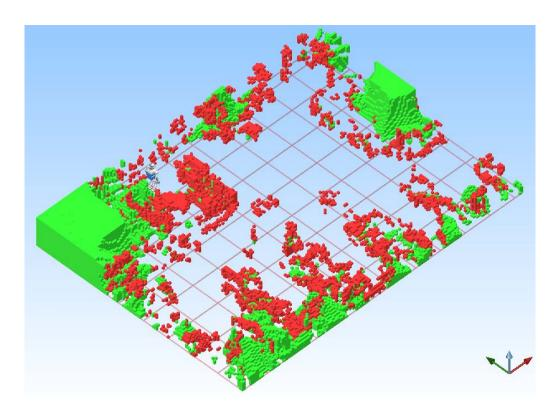
Figure 3.14: Motion planning in 3D model of robotics lab in LAAS-CNRS. The size of workspace is  $17m \times 12.5m \times 1.7m$ . The workspace is modeled with  $10cm \times 10cm \times 10cm 3D$  *Voxels*. Also, workspace is decomposed to the  $1.5m \times 1.5 \times 1.5m$  Cells to implement the approach.
