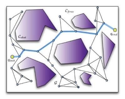
Figure 2.3: From [17]: In the PRM algorithm a roadmap  $\mathcal{R}$  is build around the obstacles by drawing random collision-free configurations (nodes) and connecting them to their nearest neighbors using feasible robot motions (edges). The query is solved by connecting  $\mathbf{q}_{init}$  and  $\mathbf{q}_{end}$  to the graph and then finding the shortest path on it (thick lines)
