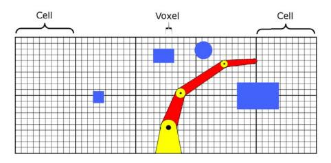
Figure 3.13: 2D cell decomposition for a robotic arm.
