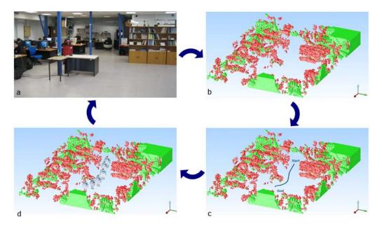
Figure 1.2: Autonomous robot in an environment: a- Perception, b- Modeling, c- Motion Planning, d- Execution.
