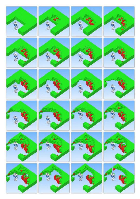
Figure 6.2: Exploration of an unknown environment. Red and green voxels represent *occupied* and *unknown* volume. The robot plans a path to the NBV after updating the model.
