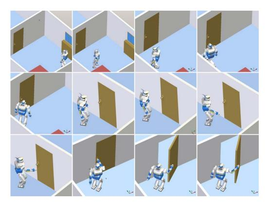
Figure 4.13: Solution path for a complete resolution of a door opening problem. The walk motion at start was generated separately with a walk planner. We then successively solved a hand reaching problem to grab the handle and a specific door constraint problem to keep the hand on a given arc of a circle.
