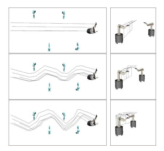
Figure 3.3: From [8]: On the left: Four manipulator arms move into the path of the Stanford Mobile Manipulator; replanning using elastic strips is performed in real-time to maintain a valid path. The path is indicated by lines connecting points on conscutive configurations along the elastic strip. It is converted into a smooth trajectory during execution. On the right: A Stanford Mobile Manipulator moves into the path of another one. The path is updated in real-time to avoid a collision.
