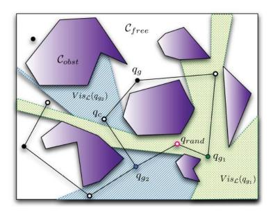
Figure 2.5: From [17]: The Visibility-PRM algorithm produces a compact roadmap around obstacles with only a few nodes: guards  $\mathbf{q}_g$  (dark circles) and connectors  $\mathbf{q}_c$  (in white). A new randomly drawn configuration  $\mathbf{q}_{rand}$  is added as a guard if it covers a previously unseen visibility domain with a given L or as a connector if it serves as liaison between at least two connected components.
