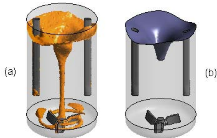
Figure 12.5. The mixing vessel with a free-surface: (a) free-surface shape calculated from an isosurface of water volume fraction equal to 0.9, N = 275 RPM, inhomogeneous approach; (b) the modified geometry with the free-surface used to cut away the gas space.
