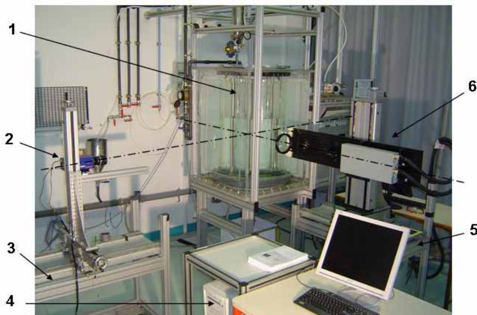
Figure 3.7. PIV apparatus on the pilot reactor: 1. mixing vessel; 2. CCD camera; 3. camera support; 4. PC and timing controller; 5. laser support; 6. laser and light optics.
