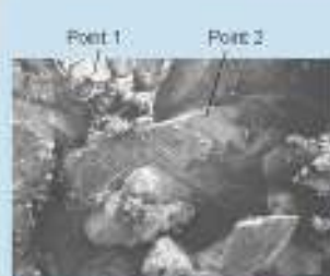
Fig 4: SEM picture and EDS spectra of Ca and Mg phosphates
