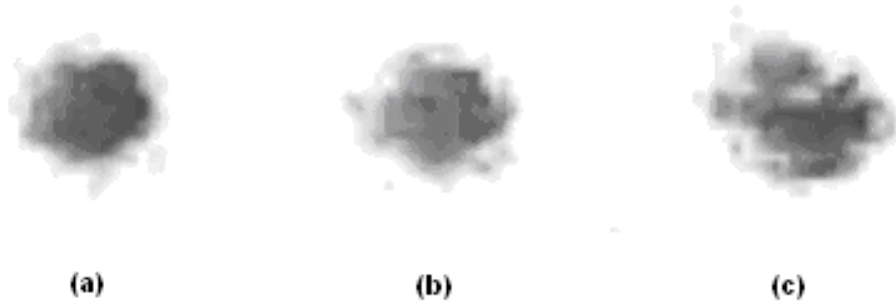
Fig. III:46 Laser beam spots on the metallic surface of the PZT that have been captured by a standard web-cam placed just outside the optical path.(a) 9 fringes, (b) 10 fringes, and (c) 11 fringes.
