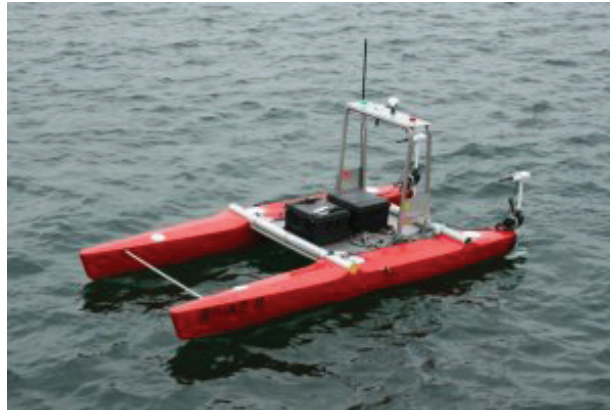
Figure 2.3 – ROAZ II : an autonomous surface vehicle used at LSA's lab
