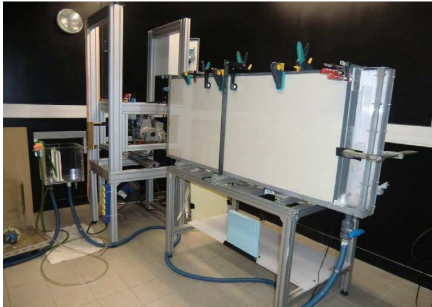
Fig. 9.1: Photo of the 2D experiment; the photo show also the tide machine used to generate the tidal forcing on the beach face.
