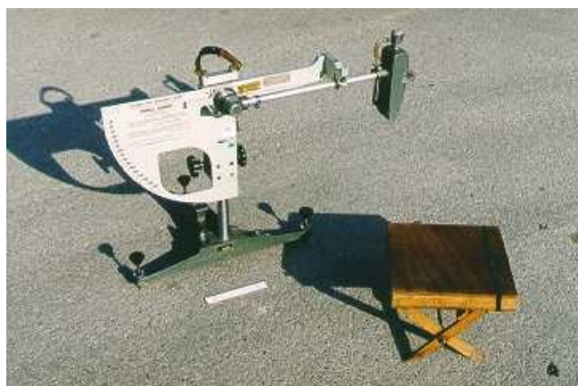
Slika 11: Prenosno nihalo SRT (arhiv ZAG) Figure 11: Portable skid resistance tester SRT (photo ZAG)
