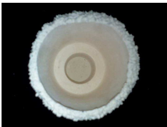
Figure 4(b) Condition of ceramic Mould after firing with clean surface without wax.
