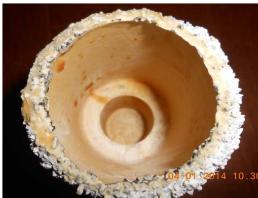
Figure 4(a) condition of ceramic Mould after dewaxing with remnant of wax.
