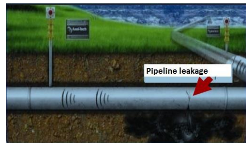
Figure 1 Crack that caused leakage
