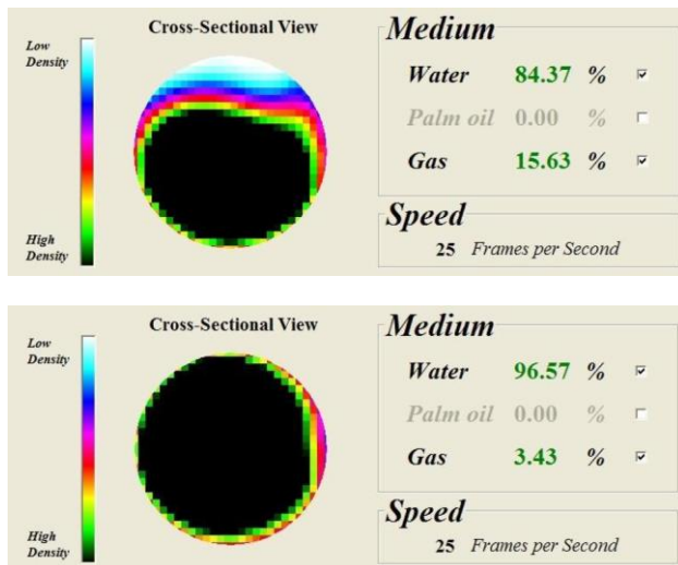
Figure 9 Reconstructed image obtained of different flow concentration of water / air two phase flow
