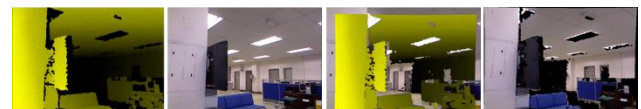
Figure 2 Shows the view of Kinect. depth data, RGB data, depth + RGB data and depth with color information (start from left)
