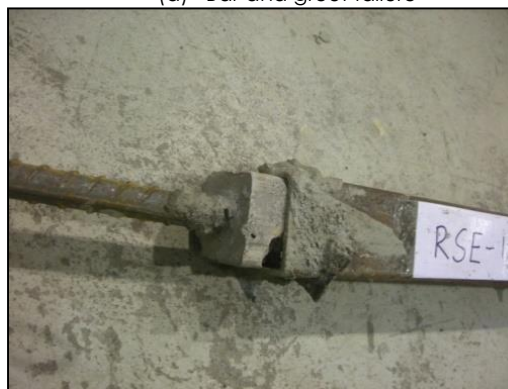
(b) Grout and sleeve failure
