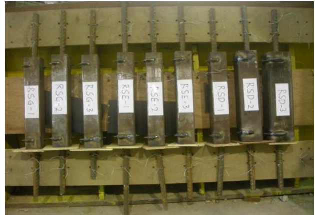
Figure 5 Pouring of Grout into Sleeves
