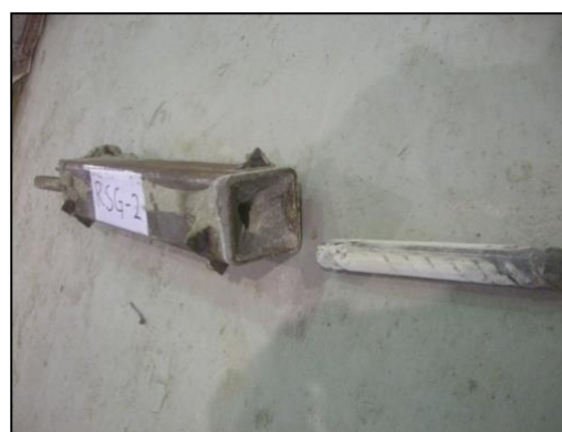
(a) Bar and grout failure
