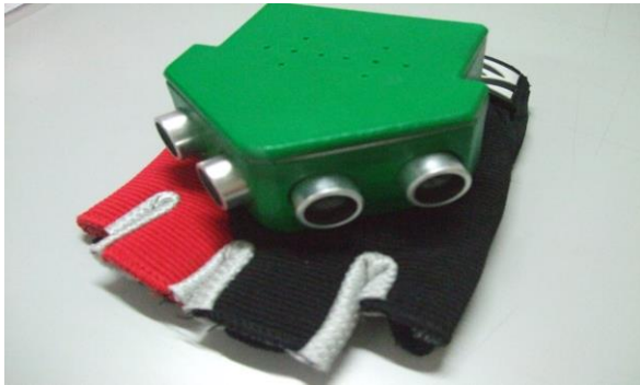
Figure 8 Final design/look of the sonar assistive device
