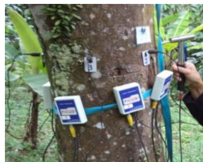
Figure 2 The set-up of acoustic tomography in agarwood imaging [3]
