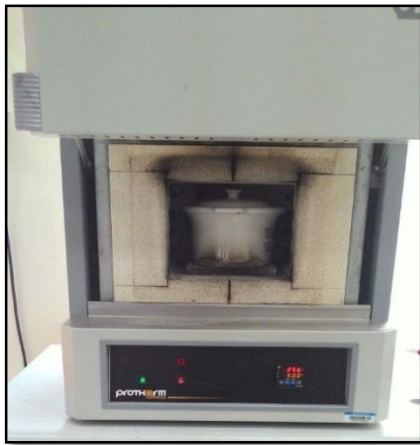
Figure 1 Sugarcane Bagasse burning process in the furnace
