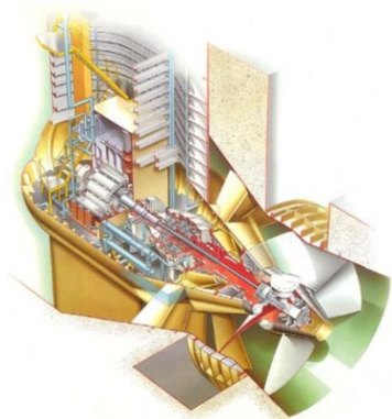
Figure 15 The bulb propeller turbine [26]
