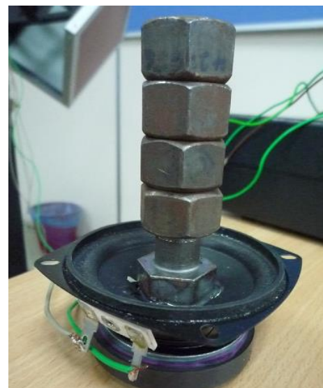
Figure 6 A photo of weights attached on the cone of a loudspeaker
