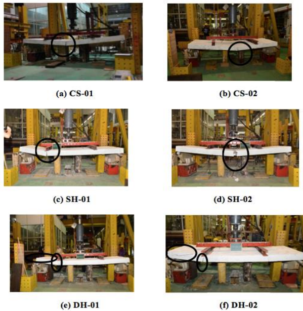
Figure 3 Failure modes for all specimens
