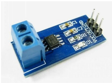
Figure 7 ACS 712 current sensor
