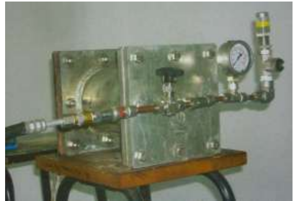
Figure 24 UTM-designed Pressurised Burn Rate Test Rig 22
