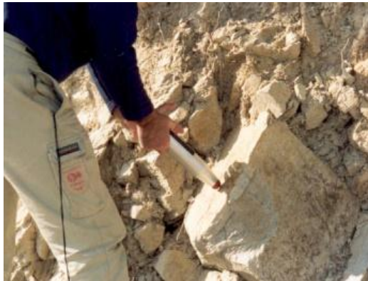
(c) Surface hardness test using rebound hammer
