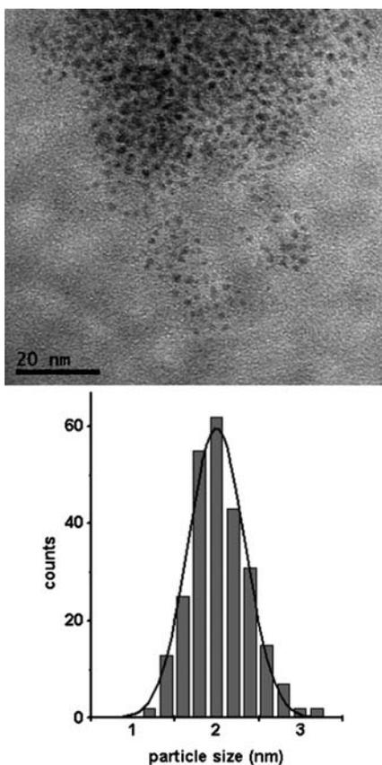
**Fig. 2** Selected TEM image of Ru(0)-NPs (2.0 ± 0.3 nm) in HM<sub>2</sub>I·NTf<sub>2</sub> and the histogram of the NPs size distribution.
