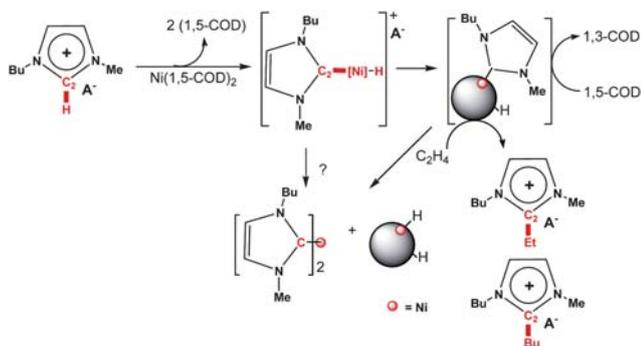
**Scheme 4** Reactions occurring during the auto-decomposition of [Ni(COD)<sub>2</sub>] in imidazolium ILs.
