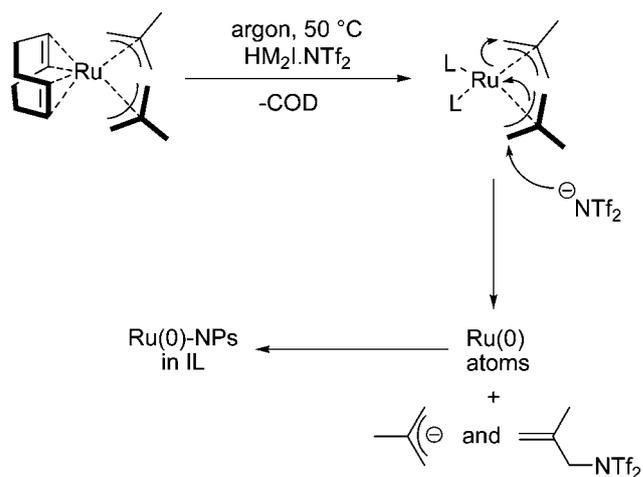
**Scheme 2** Proposed reductive elimination of the allyl-ligand induced by the NTf<sub>2</sub> anion (L = ligand/solvent-IL).
