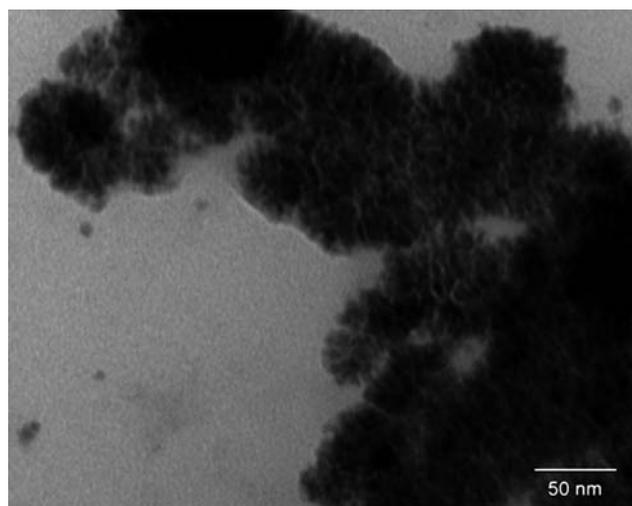
**Fig. 3** Sponge-like agglomerates of Ni(0)-NPs formed by auto-decomposition of [Ni(COD)<sub>2</sub>] in BMI·NTf<sub>2</sub>.
