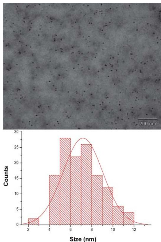
**Fig. 4** TEM image of Ni(0)-NPs (7.0 ± 2.0 nm) formed by auto-decomposition of [Ni(COD)<sub>2</sub>] in BM<sub>2</sub>I·NTf<sub>2</sub> and size distribution histogram.
