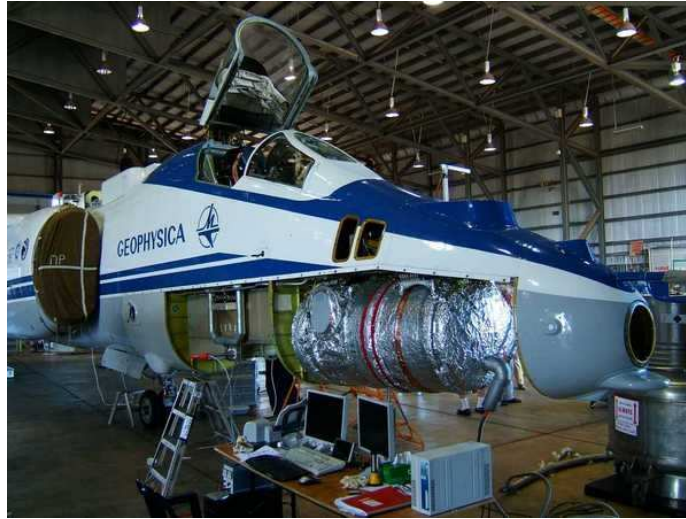
Figure 5.1: CRISTA-NF on board of the high-flying research aircraft M55 Geophysica. Source: http://www.atmos.physik.uni-wuppertal.de .
