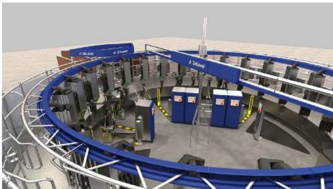
Figure 1. The AMR with 24 stations suitable for herd-sizes of 300-800 cows.
