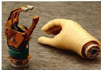
Figure 1.2: Example of myoelectric and tri-digit prosthetic hand
