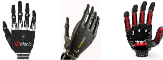
Figure 1.3: Example of polyarticular hands: iLimb, BeBionic, Vincent (from left to right)
