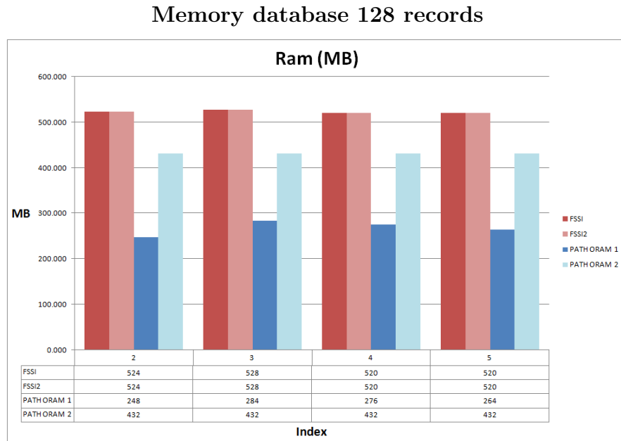
Figure 5.2: This graph shows the amount of memory required by every program after the creation on each index with a dataset of 128 records.
