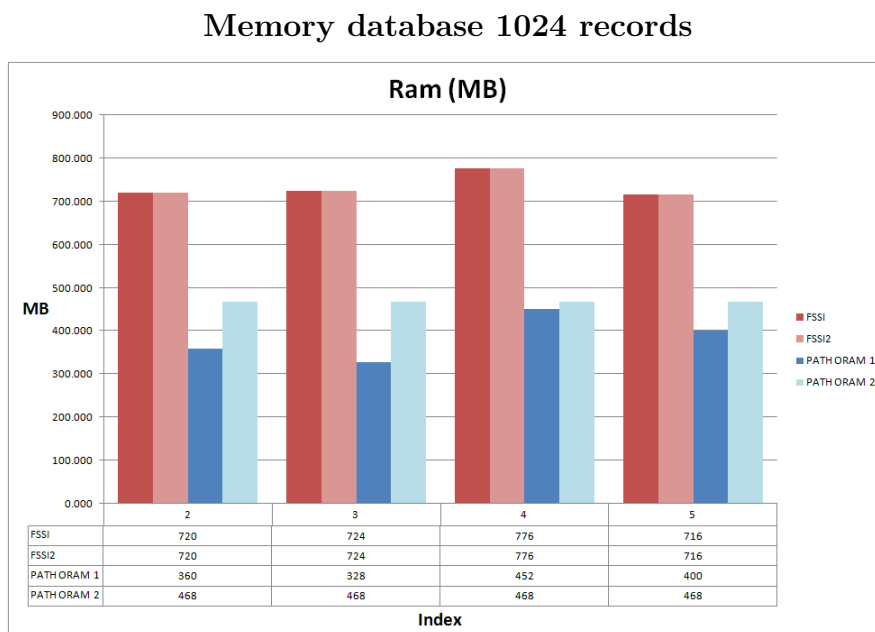
Figure 5.10: This graph shows the amount of memory required by every program after the creation on each index with a dataset of 1024 records.
