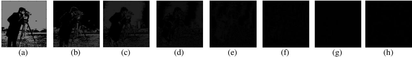
Fig. 6: Bit Plane of the image (a) - (h) is the bit-planes from highest bit to the lowest respectively
