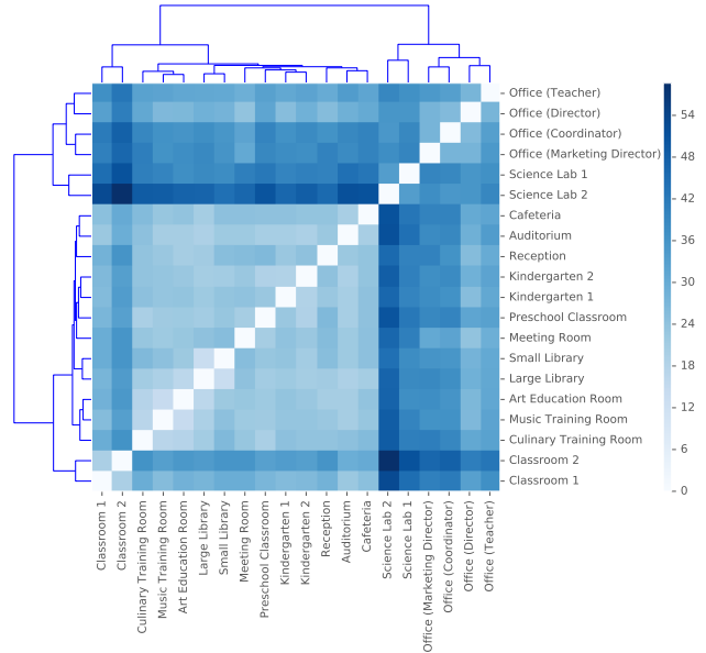
Figure 10: Agglomerative clustering on temperature movements of 20 rooms with different functionality.
