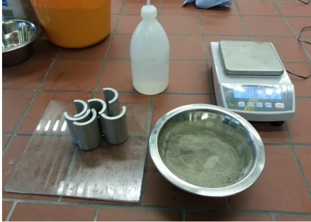
Figure 5.18. Setup for mortar samples preparation
