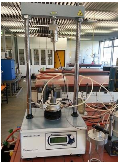
Figure 5.3. Triaxial load frame
