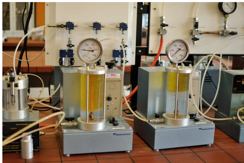
Figure 5.4. Cell and back pressure controllers
