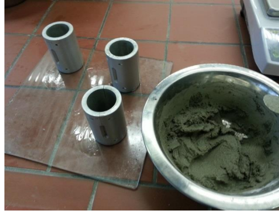
Figure 5.19. Preparation of mortar samples
