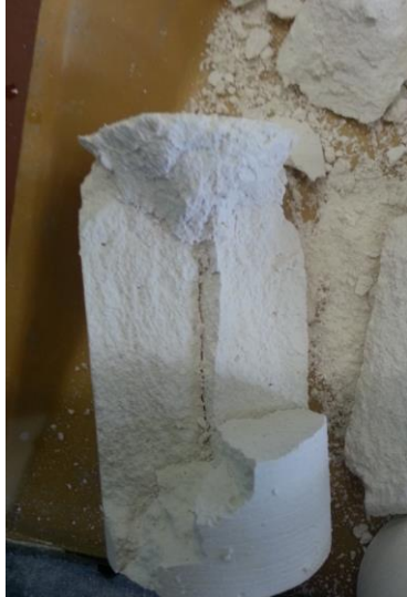
Figure 6.12. Gypsum sample after triaxial test
