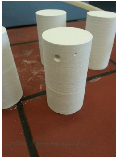
Figure B.9. Air bubbles on the surface of the sample
