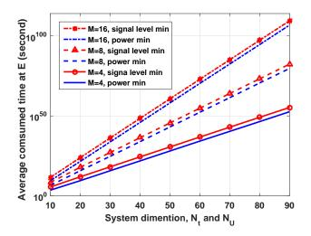
Fig. 18. Average consumed time at the eavesdropper with respect to the system dimension when using the proposed precoders with different modulation orders,  $N_e = N_t$ .
