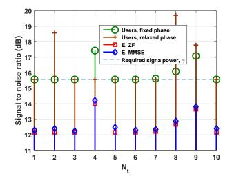
Fig. 9. Instantaneous symbol power to average noise power for power minimization precoder with fixed and relaxed phase designs when  $N_t = 11$ ,  $N_U = 10$ ,  $N_e = 16$  and  $\gamma = 15.56$  dB.
