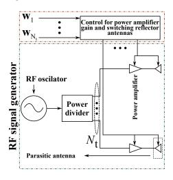
Fig. 3. RF signal generation using power amplifiers and parasitic antennas.
