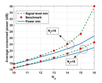
Fig. 11. Average consumed power with respect to  $N_U$  for our designed precoders and the benchmark scheme when  $\gamma = 15.56$  dB, and  $\beta^2 = 15.56$  dB.
