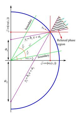
Fig. 4. Relaxed phase characterization of directional modulation design for symbol  $s_0$  from *M*-PSK modulation.
