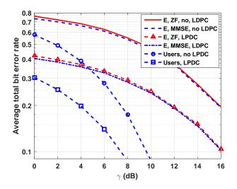
Fig. 16. Average BER versus required SNR for the signal level min precoder when  $N_t = 10$ ,  $N_e = 11$ , and  $N_U = 10$  with the code rate 5/6.
