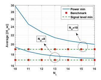
Fig. 8. Average  $\|\mathbf{H}_U \mathbf{w}\|$  for our designed precoders and the benchmark scheme when  $\gamma = 15.56$  dB, and  $\beta^2 = 15.56$  dB.
