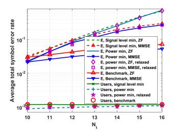
Fig. 6. Average total SER at the users and average SER at E with respect to  $N_t$  for our designed precoders and the benchmark scheme when  $N_U = 10$ ,  $N_e = 15$ ,  $\gamma = 15.56$  dB, and  $\beta^2 = 15.56$  dB.
