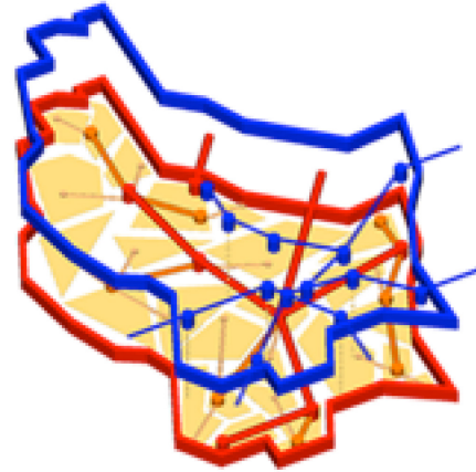
Blue: Highways with interchanges Red: Power supply network with transformers Orange: Power distribution areas
