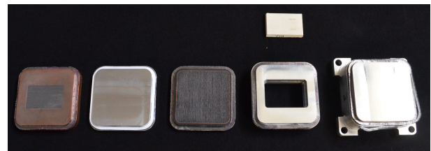
Figure 1. Injection inserts from left to right: copper encased oxy-CMC; MPIA; C/C CMC; oxy-CMC; and the laminar baseline.
