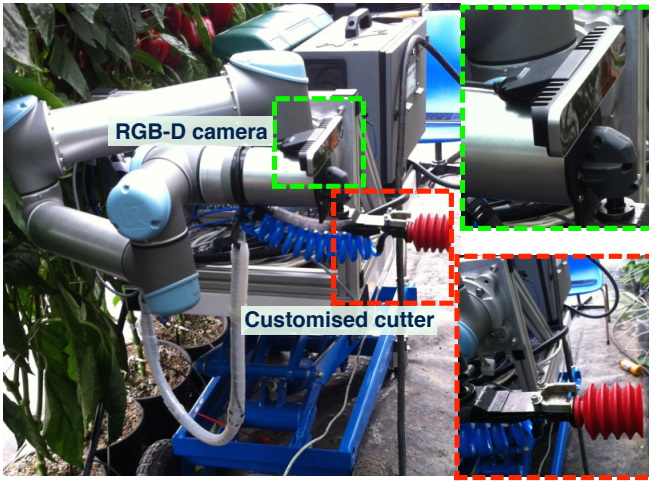
Fig. 5. QUT’s Harvey, a sweet pepper harvester prototype. In this paper, we only use the robotic arm and RGB-D sensor for peduncle detection. System integration with the proposed peduncle detection and the custom end-effector to perform autonomous sweet pepper harvesting will be tackled in future work.
