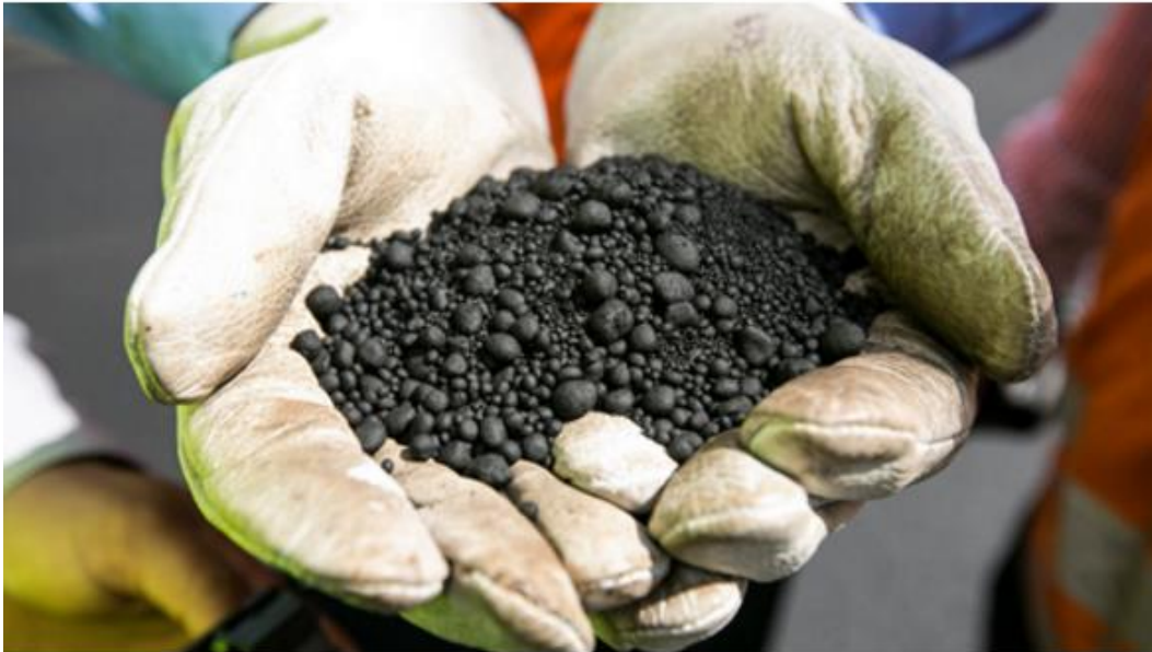
Figure 5-24: Recycled toner for road pavement
