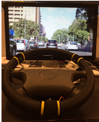
Figure 2. Simulator study setup. Each of the three touch pads was mapped to a drum sound and instructed by an LED. On the screen, the video footage of the source traffic clip was played in sync with its tracked speed-data.
