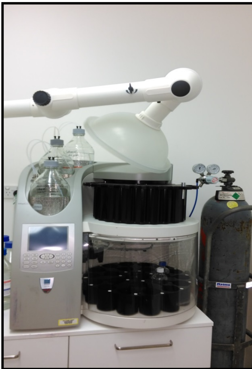
Figure 3.4 Dionex ASE 350 instrument used in extraction of target compounds in this study
