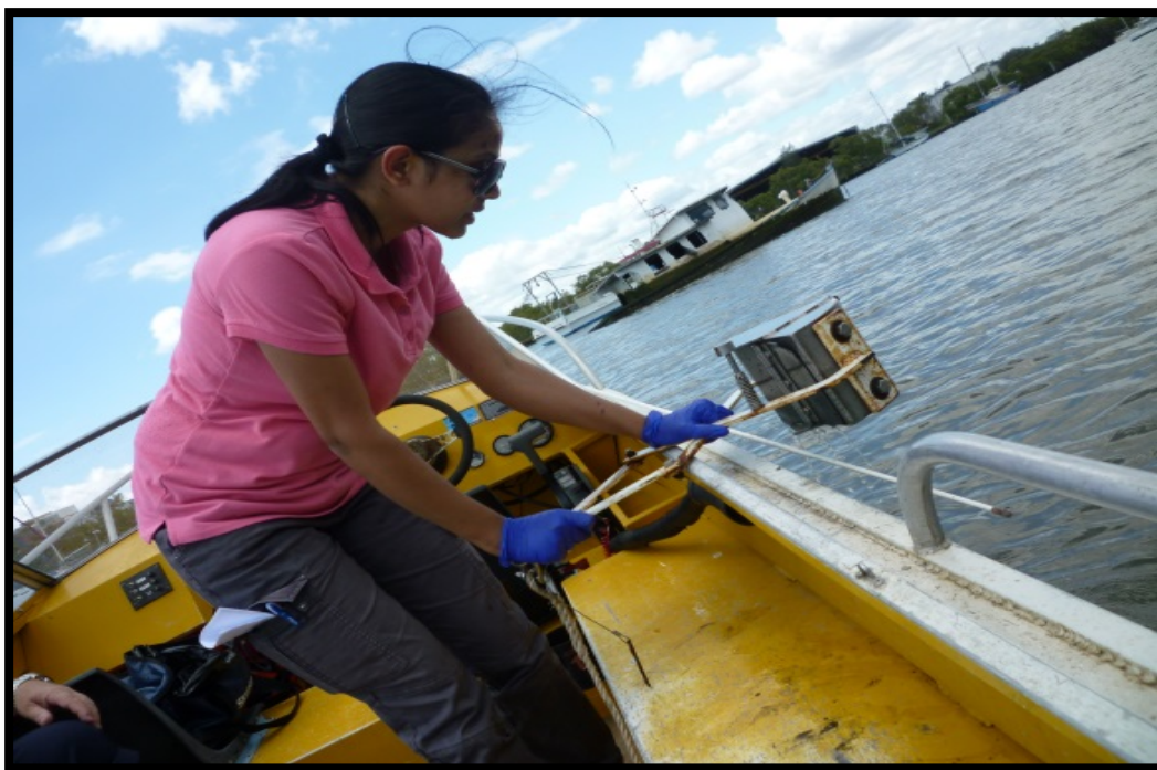
Figure 4.7 Sampling of sediment using the Van Veen Grab sampler
