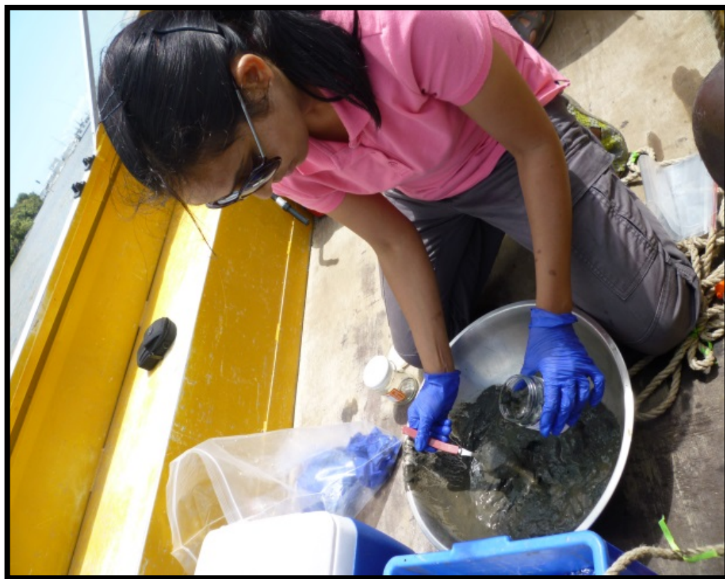
Figure 4.9 Transferring the collected sediment sample into acetone washed wide mouth glass containers
