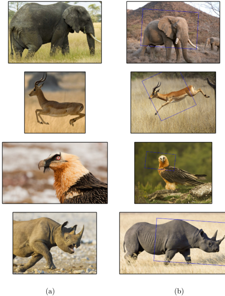
Figure 3.8: Representative pairwise alignments. (a) is the template region of interest, and (b) is the predicted region that best aligns the image to the template. The exemplars shown here all used dense SIFT features and least squares regression to learn the descent directions. The four examples exhibit robustness to changes in pose, rotation, scale and translation, respectively.
