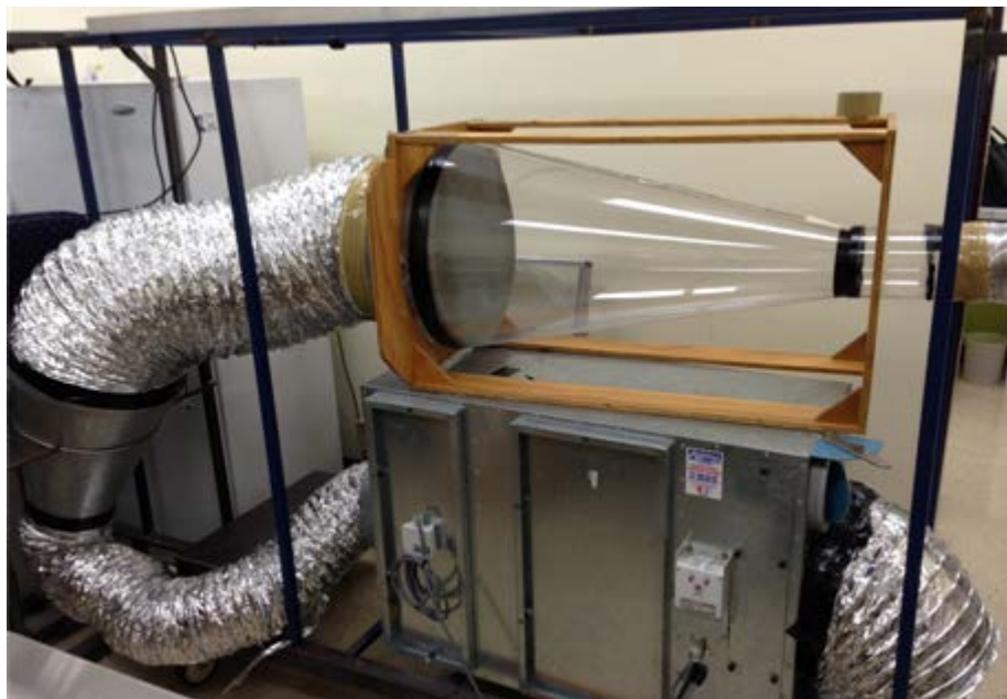
Figure 3 – HEPA filtered clean air supply.
