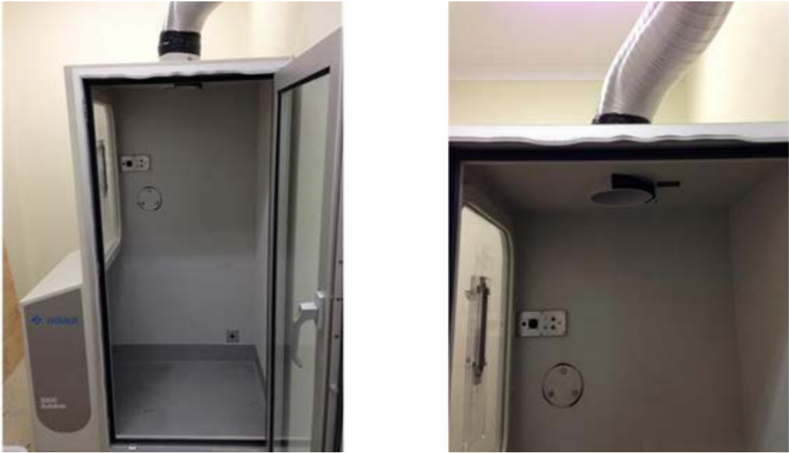
Figure 2 – Spirometry chamber and inlet.
