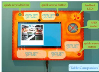
Figure 1: Prototype of a tablet companion with an RFID reader [4]
