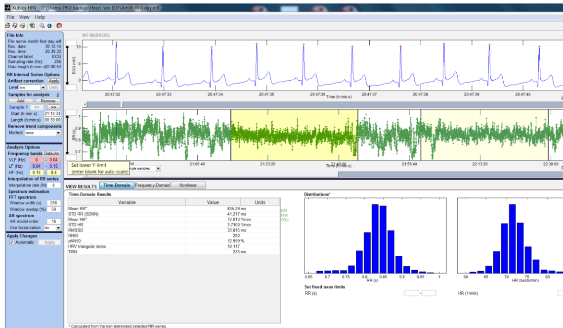
Figure 5.19. An ECG data file opened in the Kubios HRV software. The plot in green shows beat-to-beat intervals for the entire recording period. The section marked in yellow represents the sampling intervals (two driving sessions). The plot in blue (upper panel) shows the full ECG waveform sampled for R wave peak detection (peak detection marked as a red cross).
