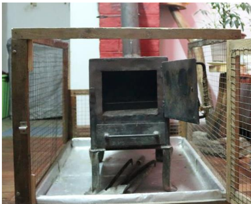
Figure 2.9: Metal chimney stove (bukhari) used for heating and usually not for cooking.
