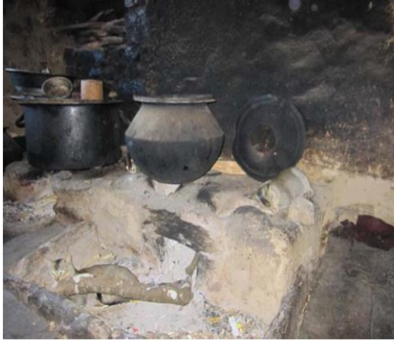
Figure 6.3: A traditional mud stove. The stove consists of one to two openings through which fuel and ash is removed, and two or three potholes, with raised lumps where pots can rest.
