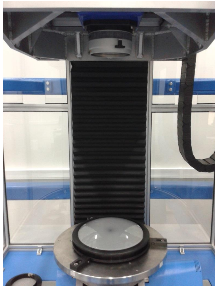
Figure 5.11: 465 mm ROC convex sphere used for Metrology Station pass-off testing
