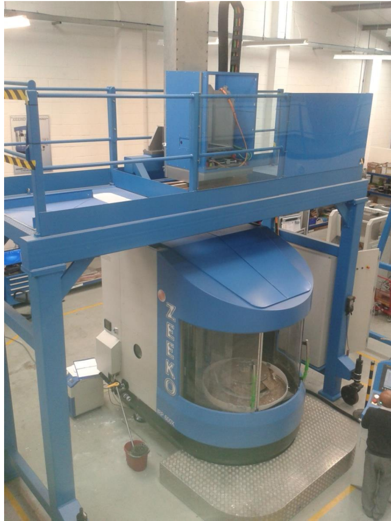
Figure 6.1: IRP600XL combined with metrology testing tower
