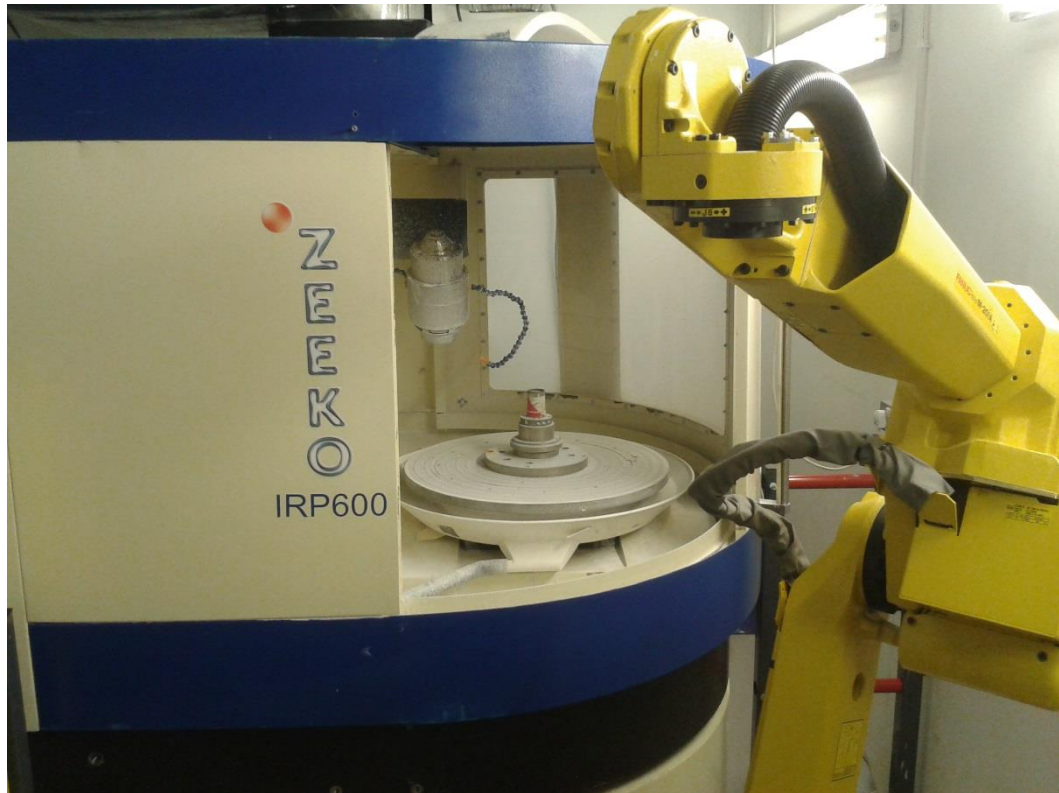
Figure 4.29: Prototype optic production cell including a Zeeko IRP600 and Fanuc M20i-A robot arm
