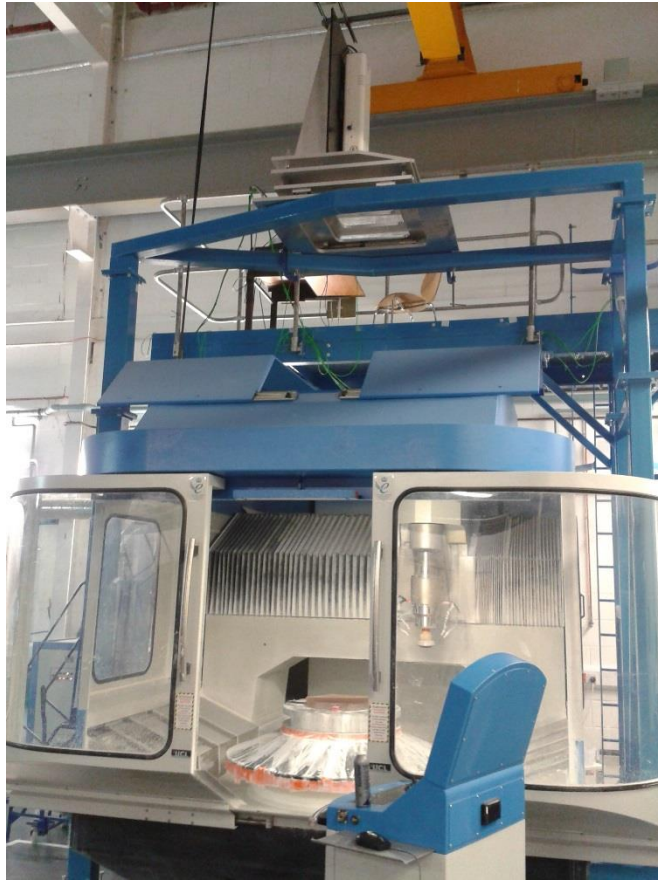
Figure 2.1: IRP1200 machine with interferometer test tower at OptIC, North Wales
