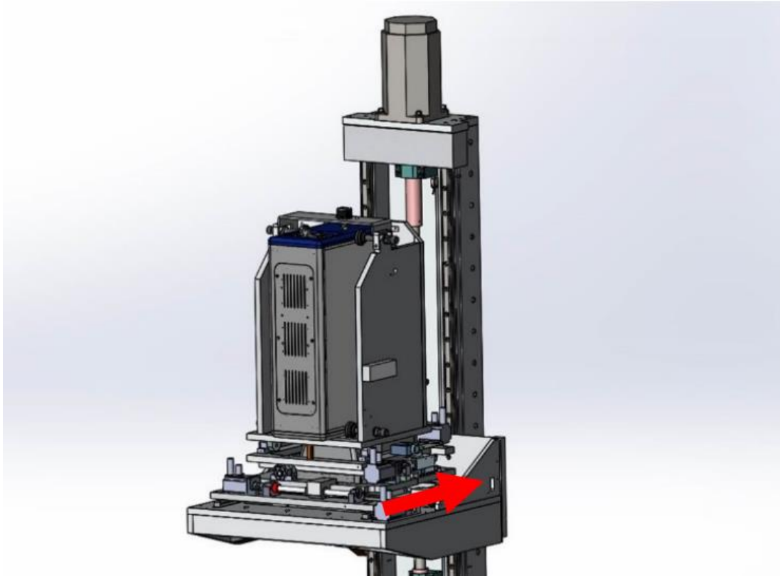
Figure 2.18: Metrology Station 5-axis stage axes configuration (courtesy of Zeeko)
