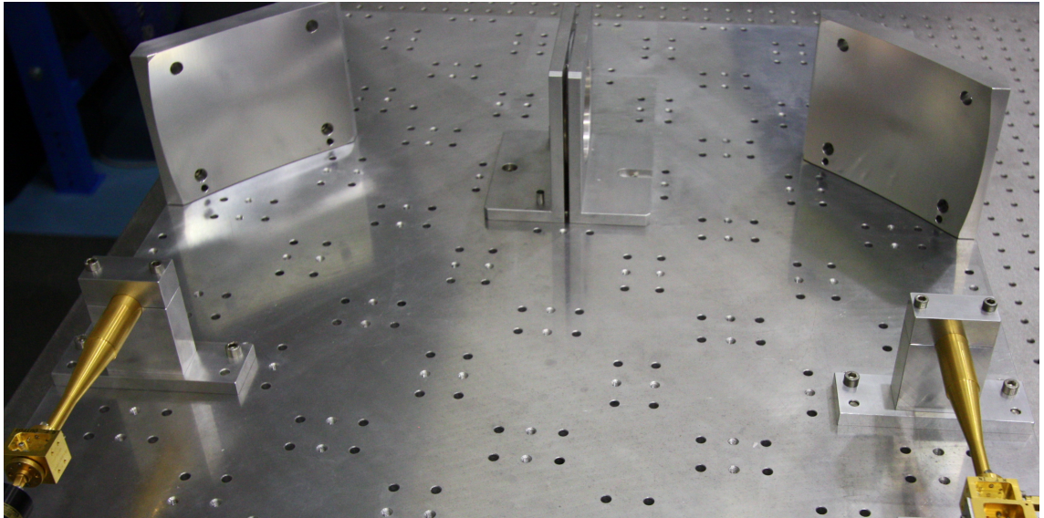
Figure 4.3: Quasi-optical test bench in transmission configuration: corrugated horns, elliptical mirrors and sample holder.
